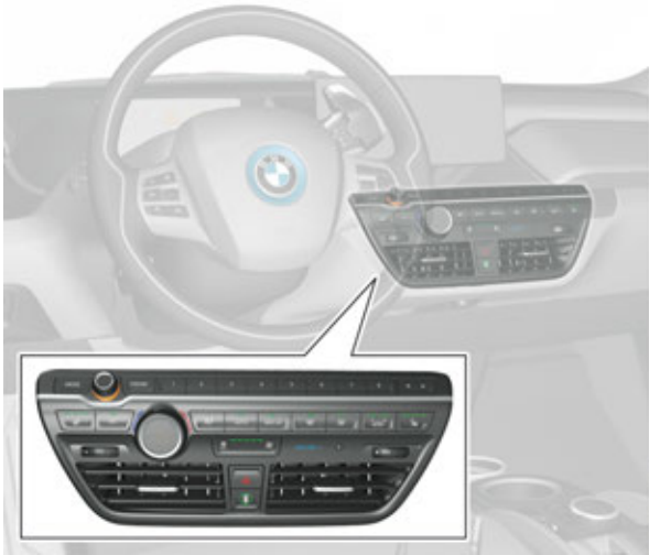
Integrated automatic heating / air-conditioning
